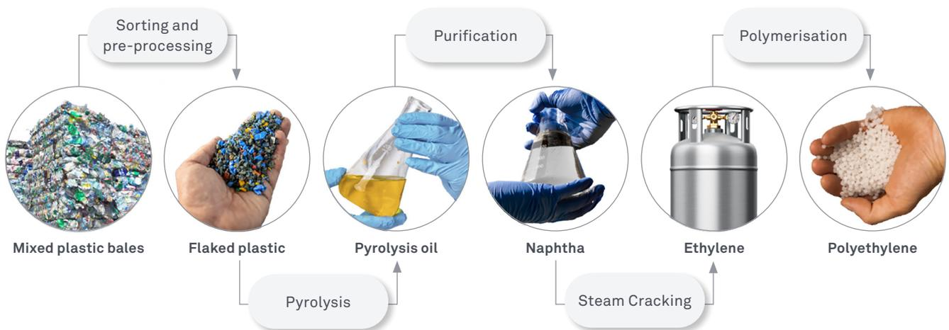
Figure 1. Process flow to chemically recycle mixed plastic waste to virgin quality polyethylene.
